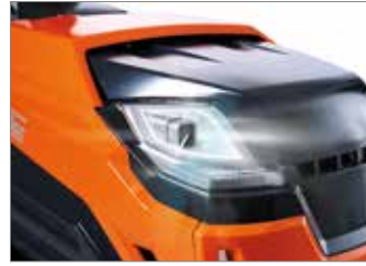
LED headlights with daytime function ensure high visibility even in low light conditions.
