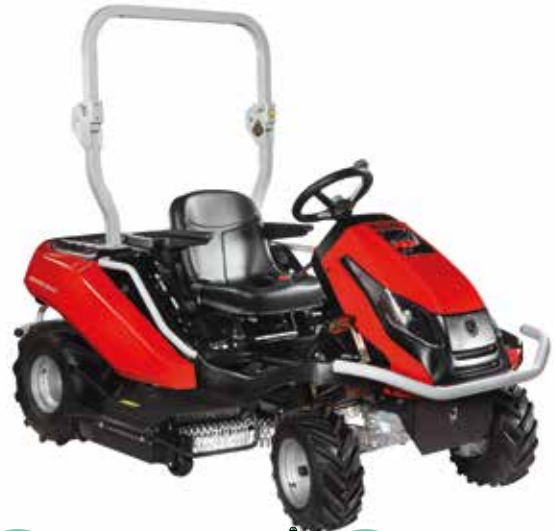
Equipped as standard with roll bar, front and rear bumpers, side guards and seat belt to ensure maximum safety, even when tackling the most complex situations ( CHEYENNE ).
