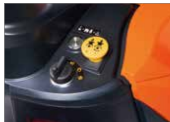
The cutting blades are activated simply by pushing the electromagnetic clutch control button located on the dashboard. This system engages the blade with no kickback.
