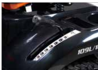
Practical cutting height adjustment with a conveniently positioned lever, with a graduated scale to show the cutting height, selected from among 7 positions.
