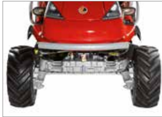
The large tyre footprint and low centre of gravity combine to maximise stability of the machine, even on steeper gradients and when working alongside verges and ditches.
