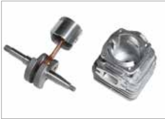
Piston with 2 rings, nickel-plated diecast cylinder, forged connecting rod and crankshaft: all features guaranteed to make the engine extremely rugged and durable.
