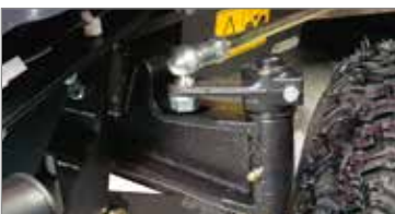
Front axle cast in steel to withstand even the heaviest of duties and resist accidental impact.
