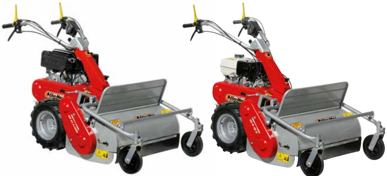
Independent steering clutches on the driving wheels with wheel locking function, making the machine extremely easy to manoeuvre.
