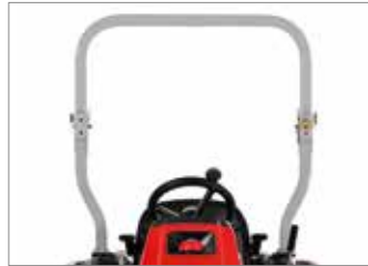
Equipped as standard with roll bar, front and rear bumpers, side guards and seat belt to ensure maximum safety, even when tackling the most complex situations ( CHEYENNE ).
