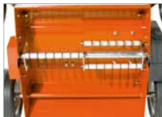
Rotor with 28 floating blades mounted on ball bearings and grease nipple system.
