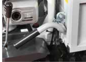
Manual dump with automatic locking system.
